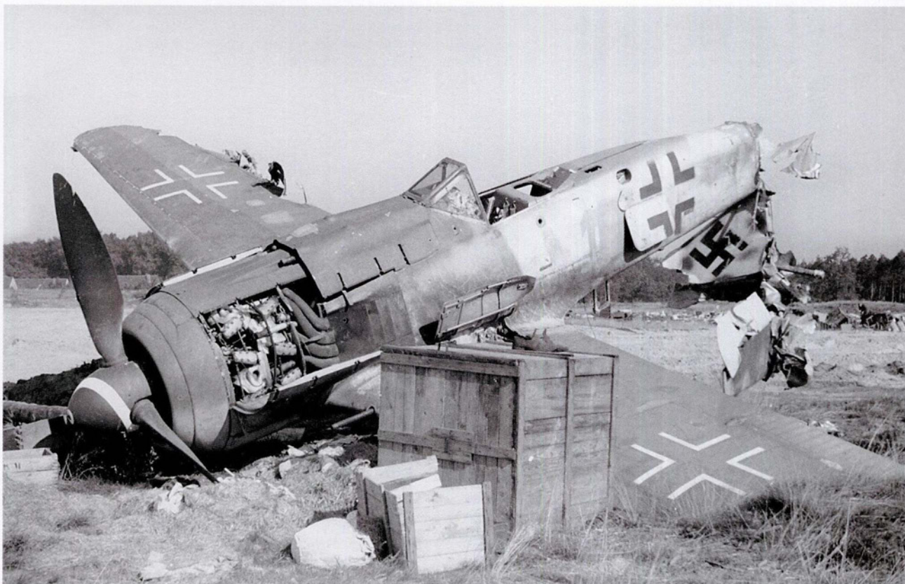
ABOVE: 'White 11' was found abandoned at Berlin-Gatow at the end of the war but was photographed in early 1946. The Werknummer 170638 confirms that this is an Fw 190 A-8 manufactured in October or November 1944 and was probably finished in 81 and 82 on the uppersurfaces with 76 on the fuselage sides and undersurfaces. Both uppersurface colours have weathered and faded so that the new 81 or 83 sprayed over the repairs on the horizontal tail unit and the starboard outer wing show as dark patches against the original colours. Note also that where the tactical number has been moved from behind the fuselage Balkenkreuz, the patch of 76 is possibly the grey-green shade.
