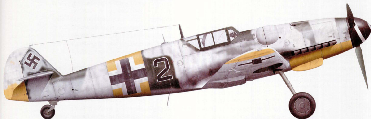
Messerschmitt Bf 109 G-6 'Black 2' flown by Uffz. Fred Schneider of 12./JG 54, Dorpat, early 1944 On this aircraft, the original 74/75/76 scheme was partially overpainted with patches of dark green, similar to RLM 71, for summer operations and then again overpainted with areas of a temporary white winter finish.
