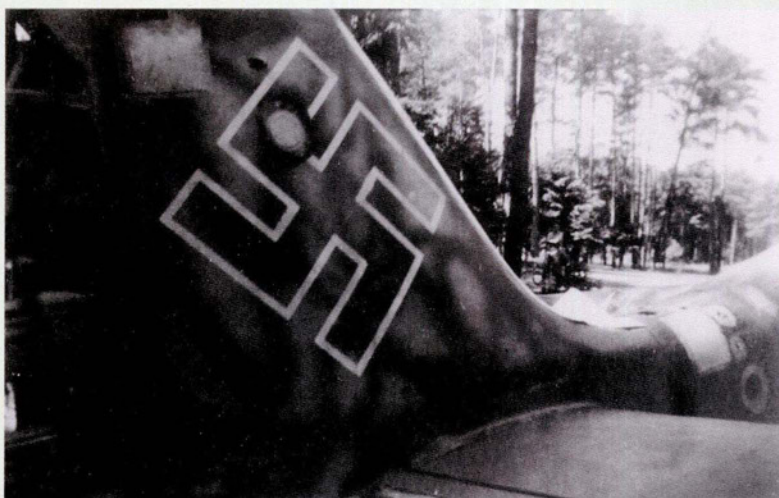
LEFT: The tail unit of an Fw 190 F-8 showing a similar dark finish oversprayed with spots of a lighter colour.
