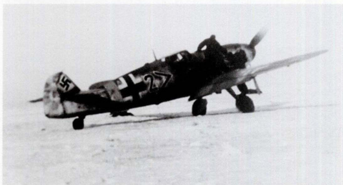
ABOVE: A Bf 109 G-6 of the Gruppenstab of I./JG 52 in the winter of 1943/44 about to start its engine. While one member of the ground crew stands on the starboard mainwheel tyre, another is on the wing and both have hold of the handle for winding the inertia starter.
