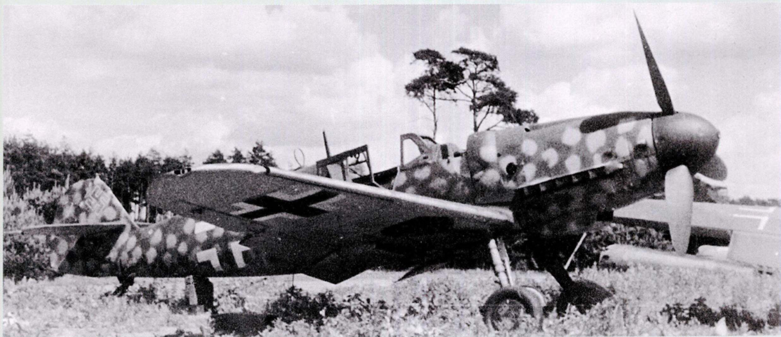
BELOW: This view of a Bf 109 G-6 or G-14 at Wunstorf shows the overall dark finish with light coloured mottling which extends well down the fuselage sides to include the area below the exhausts where the spots become darker against the undersurface colour.
